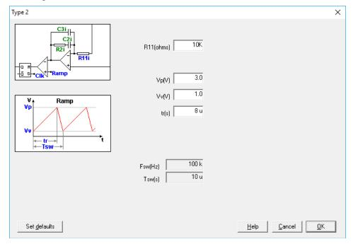
Figure 8: Type 2 inner current loop configuration
