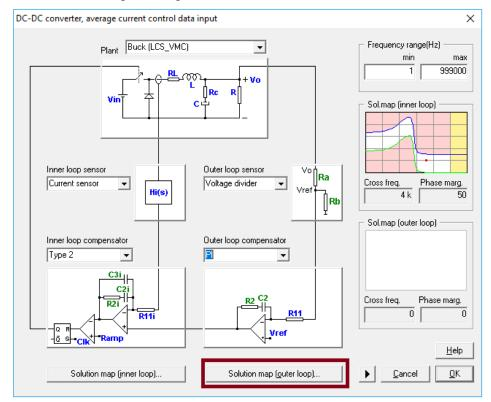
Figure 17: Select the outer loop solution map
