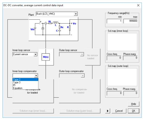
Figure 7: Selecting a Type 2 controller
