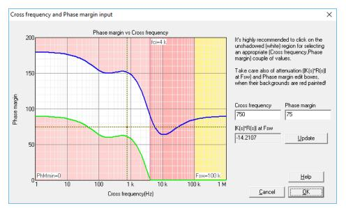
Figure 18: outer loop solution map
