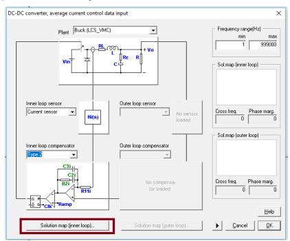
Figure 9: Access to the inner loop solution map
