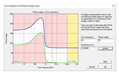
Figure 10: solution map for the inner loop
