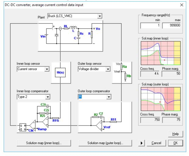
Figure 19:Double loop buck controller fully defined
