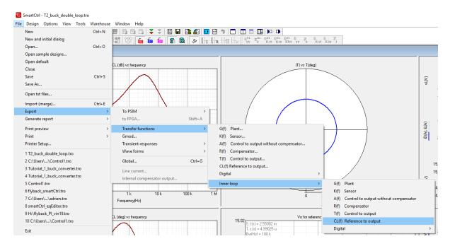
Figure 29: Exporting inner current close loop transfer function plotted
