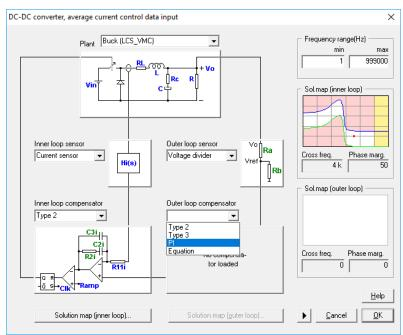
Figure 15: list of available outer loop compensators
