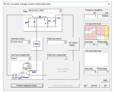
Figure 11: inner current loop fully defined
