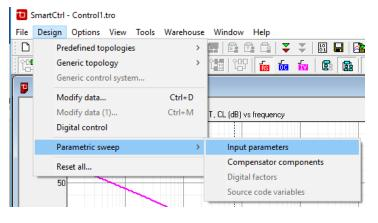
Figure 21: Accessing the parameter sweep capability
