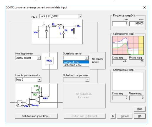
Figure 13: Outer loop sensor list
