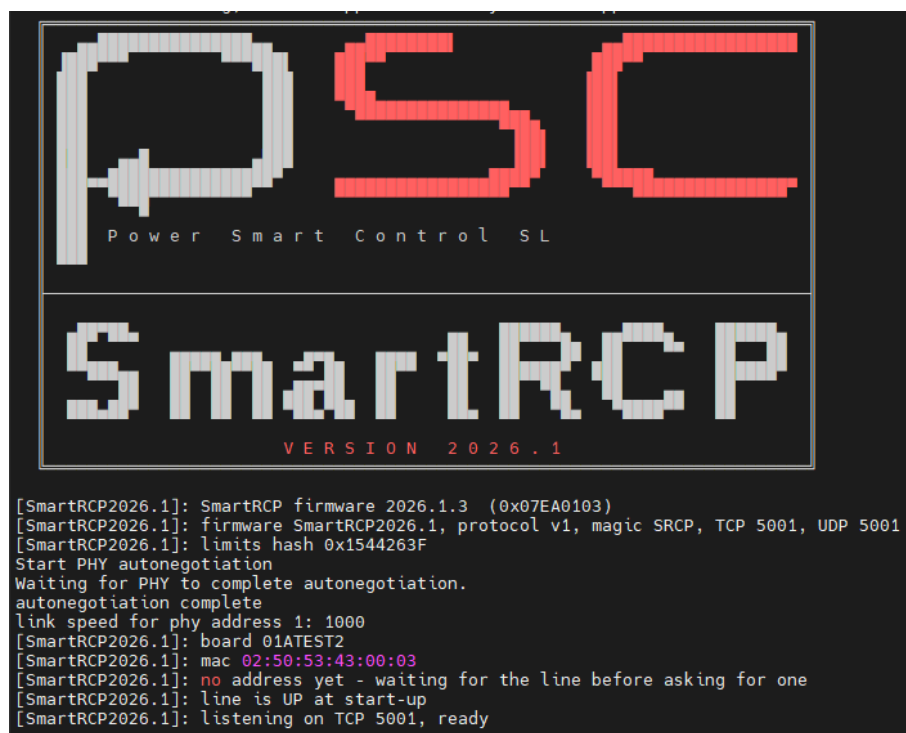
Figure 3: What the board prints on its serial console when it starts.
